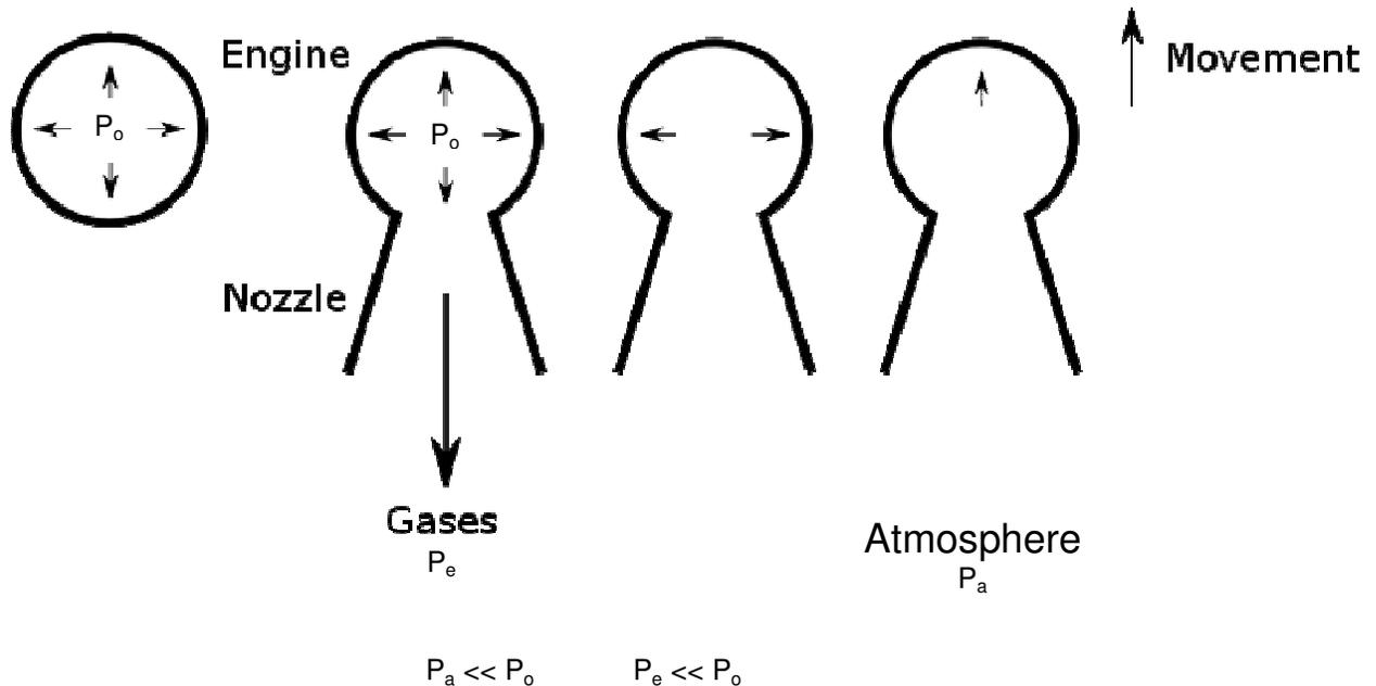
**Figure 1. Rocket engine thrust diagram**
